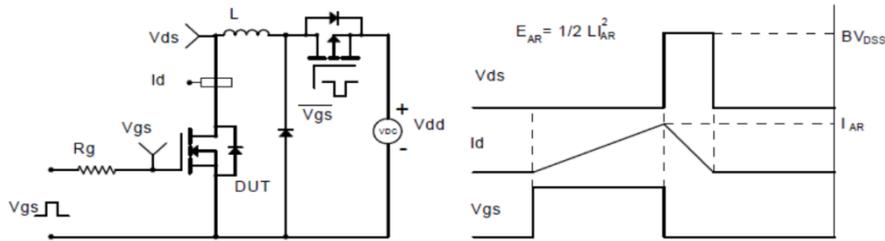
**Switching Time Test Circuit and Waveforms(N-Channel)**
